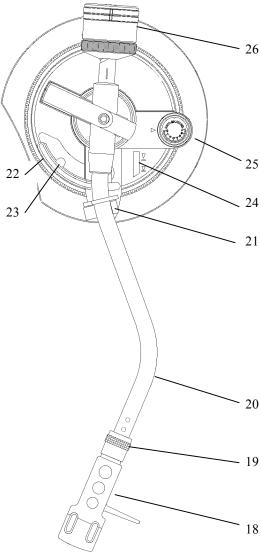
18. Headshell- Install cartridge here. When installing a cartridge, refer to the installation instructions supplied by the manufacturer of that cartridge. During installation, attach the stylus protector to guard the stylus tip from damage.
