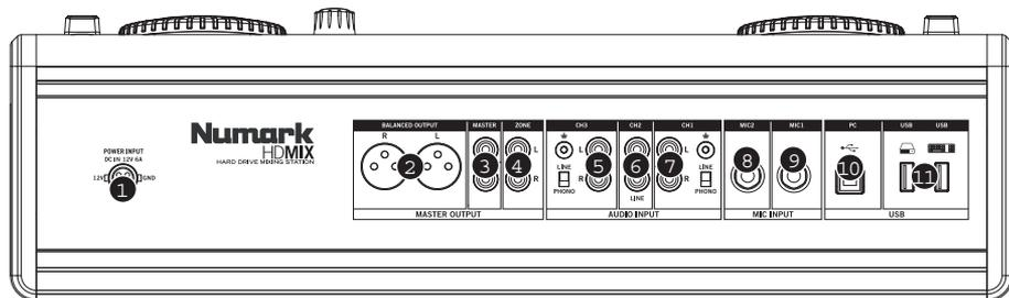
1. **Power** – Please plug in the supplied power adapter (DC 12V 2A) and connect it to a power source. Please *only* use the supplied power adapter – using an alternate power adapter may result in damage to the HDMIX.
