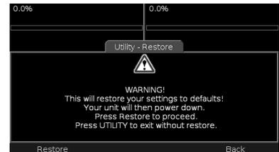
Note that the calibration (see below) will not be reset by this operation.
