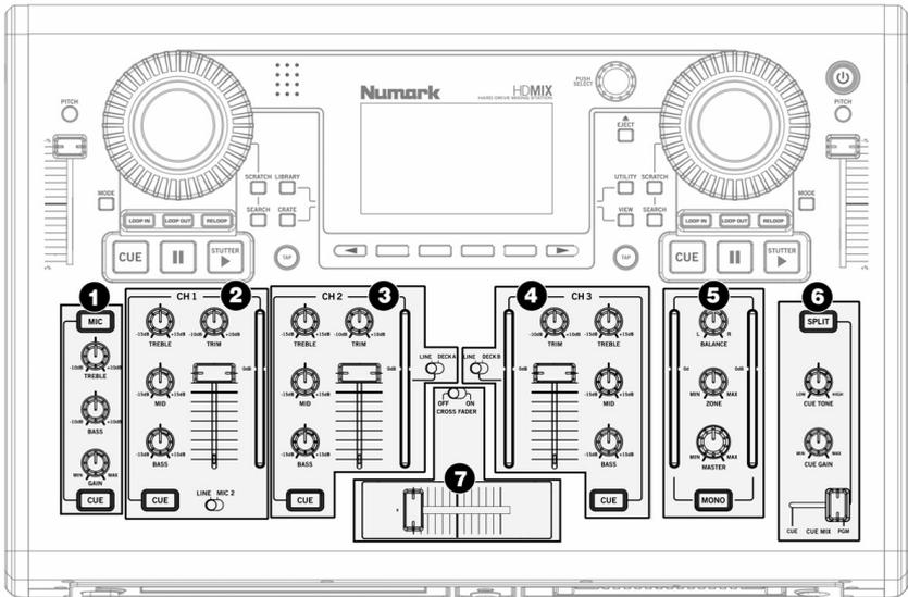
1. **MICROPHONE CHANNEL** – This channel features the following microphone controls, which affect the Mic 1 input signal. Please note that the microphone signal is not routed to the crossfader and will be sent directly to the master mix.
