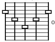
Below is an example of a poor EQ curve because it cuts the output volume down by 6-10dB. You have to compensate by running the **Master** output higher:
