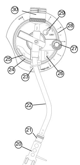
20. Headshell - Attach the cartridge here.
