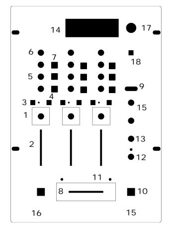
4. **Send Buttons** are for allowing a channels pre-fader output to be sent to the send connectors in the rear of the unit. These are used for sampling and other special effects. You would return the send signal through another input channel.
