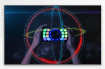
Built-in two-axis accelerometer allows manipulation of effects and filters by tilting forward, back, left, or right.
